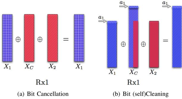
Fig. 3. Basic transmission techniques at the cognitive relay.
