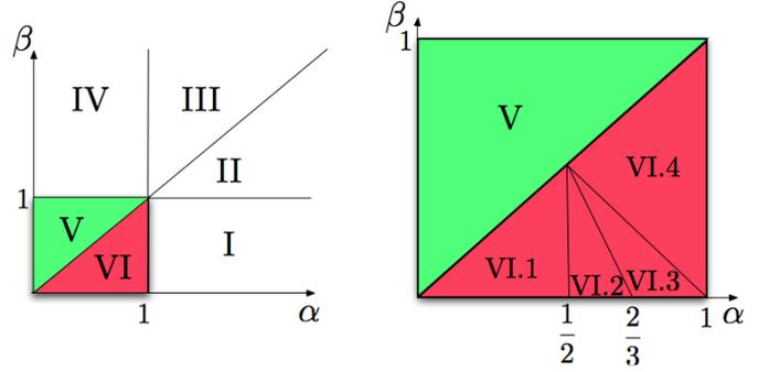
Fig. 2. Regimes of operation for the linear deterministic IFC-CR, where  $\alpha := n_I/n_S$  and  $\beta := n_C/n_S$ .
