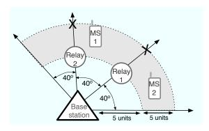
Fig. 3. Geometric distribution: relays at equal distance, spaced at angles  $40^{\circ}$  on arc of radius 5 units, mobiles random in shaded sector for the *random MS* placement, or at the points marked X for the *fixed MS* placement.
