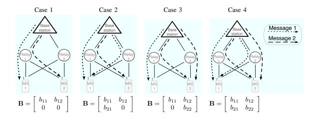
Fig. 2. Four message knowledge scenarios when  $|h_{BR_1}| \ge |h_{BR_2}|$ , and the corresponding linear precoding matrices **B**.
