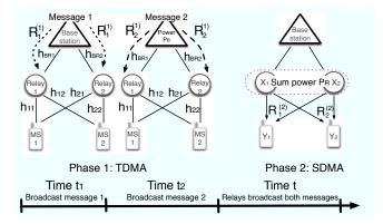
Fig. 1. Transmission takes place in two phases: in phase 1 the BS broadcasts messages in TDMA fashion: message  $W_1$  for  $t_1$  time units, then message  $W_2$  for  $t_2$  time units. During phase 2 the relays simultaneously transmit all received messages to the mobiles. Illustrated are the channel gains, power constraints, rates, and input-output variables.
