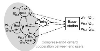
Fig. 1. Our physical channel model consists of multiple independent bi-directional desired communication flows (indicated by arrows) between multiple terminal nodes, a single relay node, and a single base-station.  $W_{i,j}$  denotes the message from node i to node j, while  $\tilde{W}_{i,j}$  is the estimate at node j of the message  $W_{i,j}$ .
